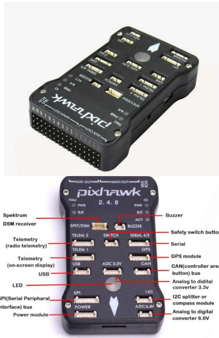
Figure 4. PX4 is an open-source professional autopilot (flight controller software) for drones. It enables autonomous control, stable flight, GPS-based mission execution, and integration of various types of sensors.
