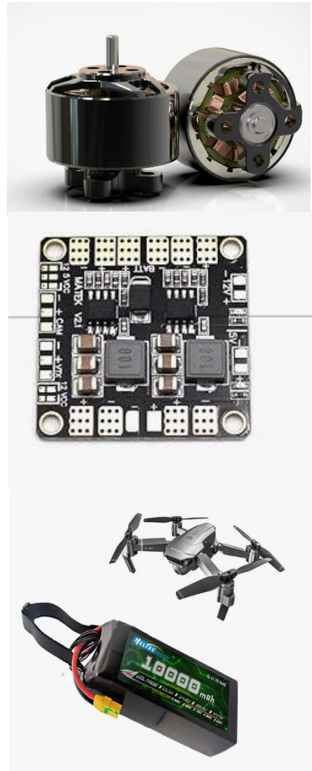
Figure 3. Power Distribution Board (PDB) and Li-Po battery. For drones, battery capacity is selected in the range of 3000 mAh to 10000 mAh depending on the UAV mission requirements.
